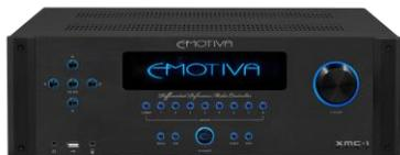
Emotiva spared no expense in designing this upgrade to make the XMC-1 the best AV processor at its price point. Eight HDMI inputs and dual HDMI outputs deliver a bit-perfect video stream, with full support for HDMI 2.0b and HDCP 2.2, and all current 4K HDR10 video formats
