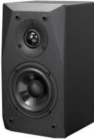
Both the **BasX LCR** (SRP: \$149/speaker) and **BasX Sat** (pictured left; SRP: \$99/speaker) models are two-way speakers featuring a ferro-fluid cooled 1" silk dome tweeter, a long-throw 4" mid/bass driver with a mineral-filled polypropylene cone and rubber surround, and a rear-firing tuning port. In addition, both models can be placed vertically or horizontally for maximum flexibility.
